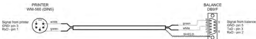
Cable: balance – KAFKA printer
