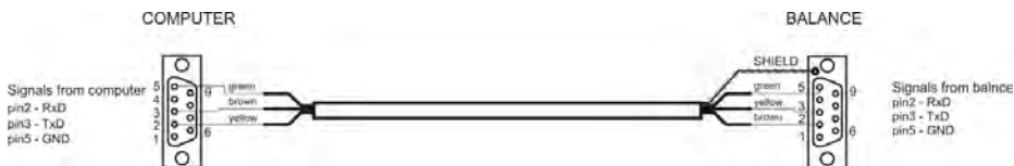
Cable: balance – computer (RS232)
