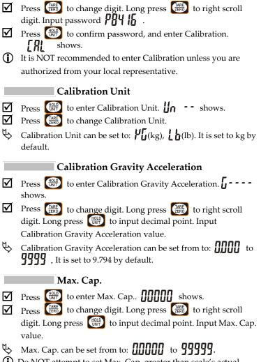
(i) Do NOT attempt to set Max. Cap. greater than scale's actual capacity. Overloading causes severe harm to scale, and is very
